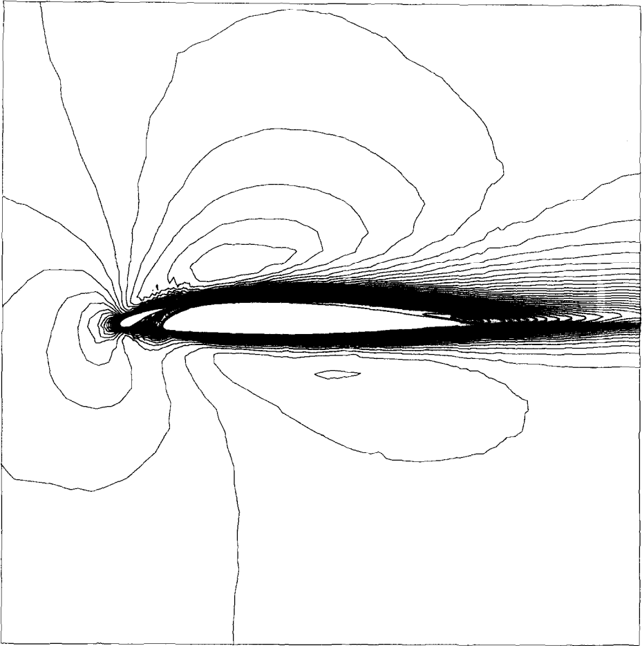
FIG. 9. Mach contours in the flow-field obtained with the Navier-Stokes solution on the initial coarse mesh for the two-element airfoil configuration, Mach = 0.5, incidence = 3^\circ , Re = 5000 .
